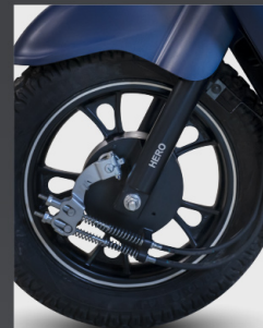
Regenerative Braking & Telescopic Suspension
